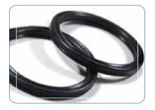
Quad rings / X-rings can be used in a wide variety of static and dynamic sealing applications. With 2 sealing areas per side for more effective sealing, quad rings have the same dimensions as the BS1806 O-ring sizes.
